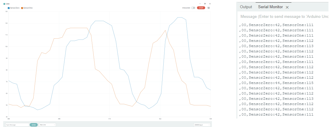
Figure 4.1.1 and 4.1.2: Serial Plot and Serial Monitor values of sensors zero and one as the disk rotated.
