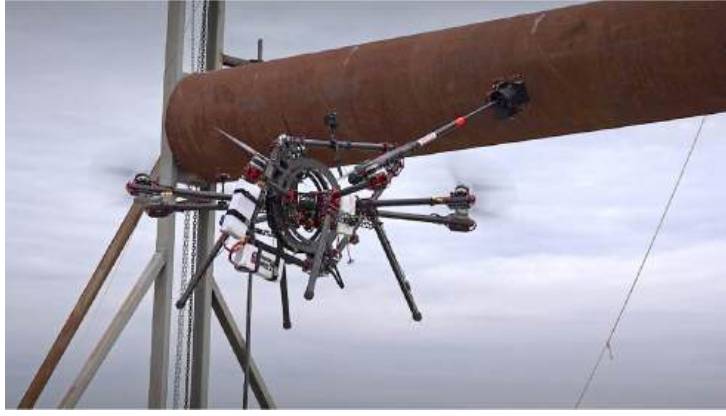
Figure 3 AeroX, a multi-directional thrust octo-rotor with an inspection arm [8]
