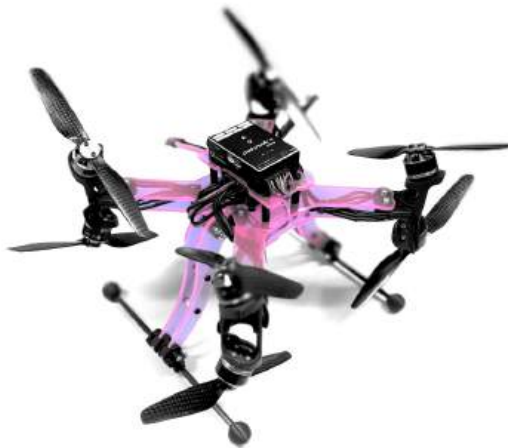
Figure 9 Prototype of the FT-X8 - a compact fixed-tilt octo-rotor [14]
