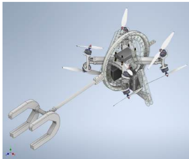
Figure 13 CAD model of the updated prototype, containing 3D models for printing and parts for laser cutting
